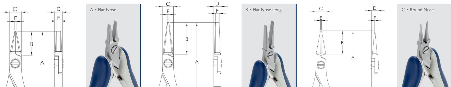
**A. - B.** flat nose pliers feature a very fine tip, smooth or serrated jaws and inner edges **C.** round nose pliers have jaws formed by two cones. A round nose pliers is generally used both to clamp and to form loops on leads or wire.
