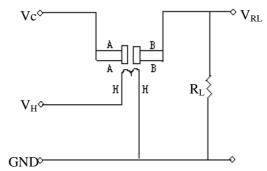
The above is basic test circuit of the sensor.
