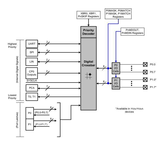
Figure 1.9. Port I/O Functional Block Diagram
