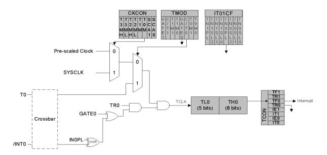
Figure 19.1. T0 Mode 0 Block Diagram
