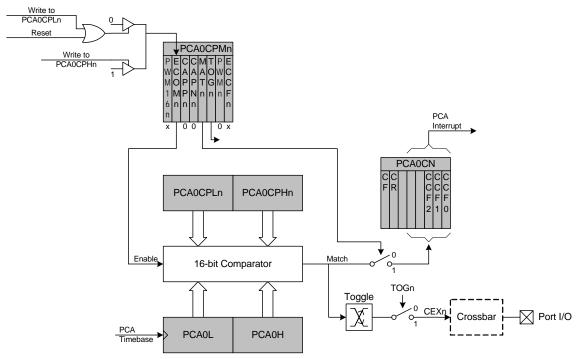
Figure 20.6. PCA High-Speed Output Mode Diagram
