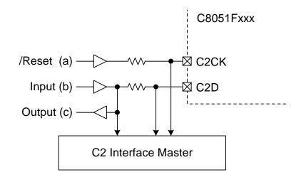
Figure 22.1. Typical C2 Pin Sharing
