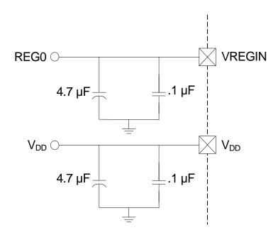
Figure 7.1. External Capacitors for Voltage Regulator Input/Output
