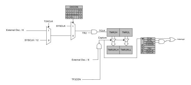
Figure 19.6. Timer 2 Capture Mode Block Diagram
