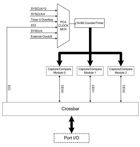
Figure 20.1. PCA Block Diagram
