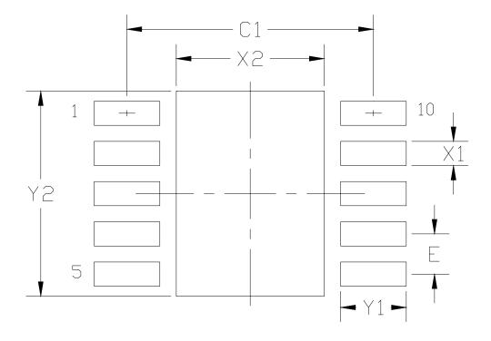
Figure 4.2. DFN-10 Landing Diagram
