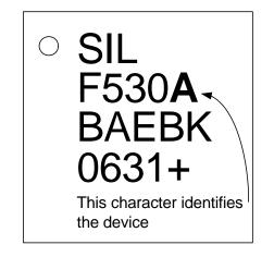
Figure 21.2. Device Package - QFN 20
