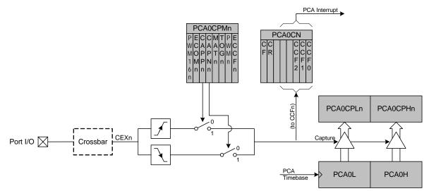
Figure 20.4. PCA Capture Mode Diagram
