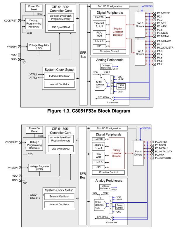
Figure 1.4. C8051F52x Block Diagram
