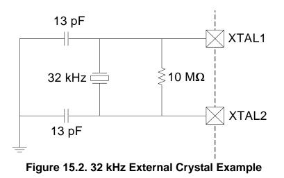
**Important Note on External Crystals:** Crystal oscillator circuits are quite sensitive to PCB layout. The crystal should be placed as close as possible to the XTAL pins on the device. The traces should be as short as possible and shielded with ground plane from any other traces which could introduce noise or interference.
