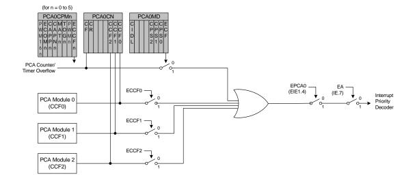
Figure 20.3. PCA Interrupt Block Diagram
