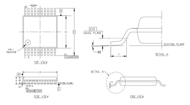
Figure 4.3. TSSOP-20 Package Diagram
