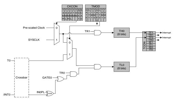
Figure 19.3. T0 Mode 3 Block Diagram
