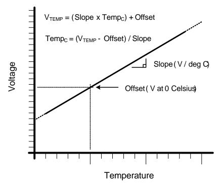
Figure 5.2. Typical Temperature Sensor Transfer Function
