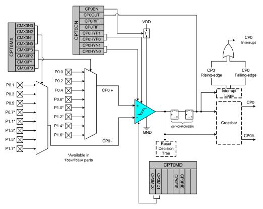
Figure 8.1. Comparator Functional Block Diagram
