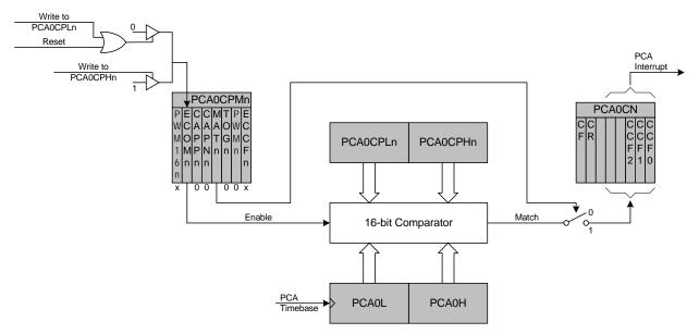
Figure 20.5. PCA Software Timer Mode Diagram
