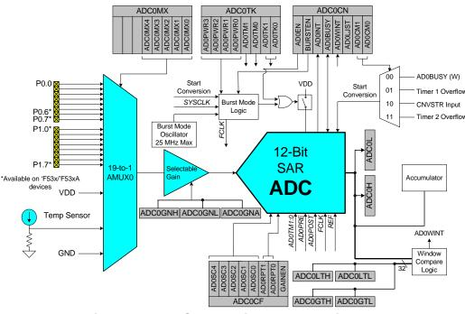
Figure 5.1. ADC0 Functional Block Diagram
