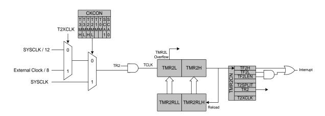
Figure 19.4. Timer 2 16-Bit Mode Block Diagram
