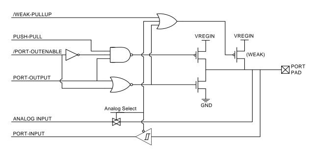
Figure 14.2. Port I/O Cell Block Diagram
