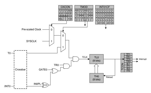
Figure 19.2. T0 Mode 2 Block Diagram
