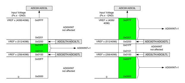
Figure 5.7. ADC Window Compare Example: Right-Justified Single-Ended Data
