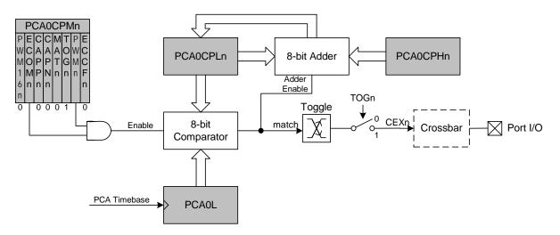
Figure 20.7. PCA Frequency Output Mode
