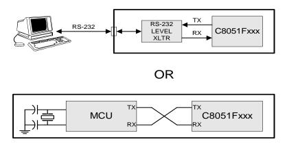
Figure 16.3. UART Interconnect Diagram
