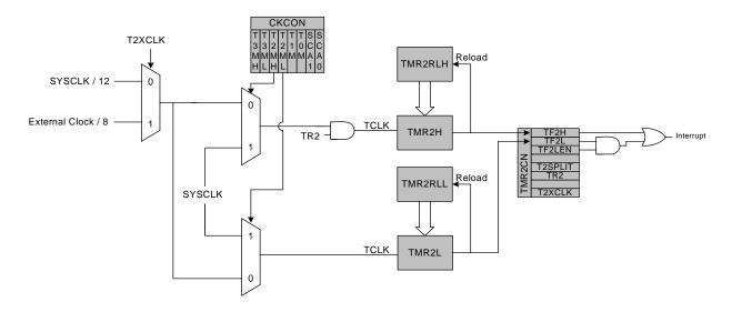
Figure 19.5. Timer 2 8-Bit Mode Block Diagram
