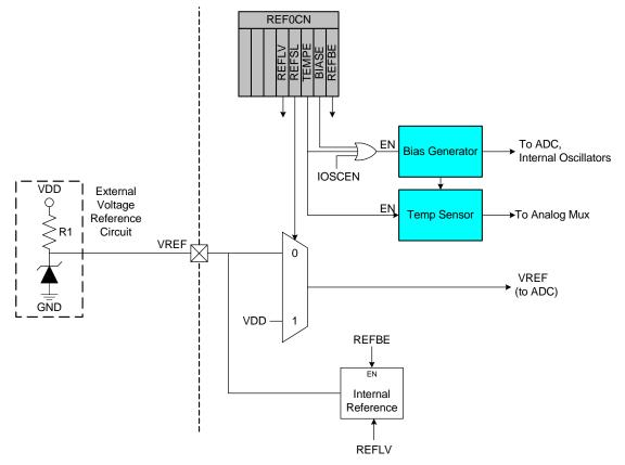
Figure 6.1. Voltage Reference Functional Block Diagram
