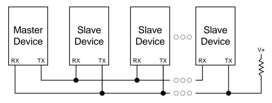
Figure 16.6. UART Multi-Processor Mode Interconnect Diagram
