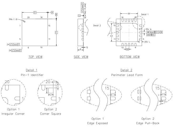
Figure 4.5. QFN-20 Package Diagram\*
