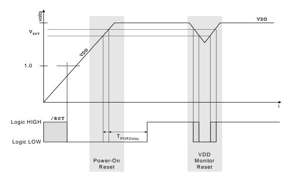
Figure 12.2. Power-On and V<sub>DD</sub> Monitor Reset Timing
