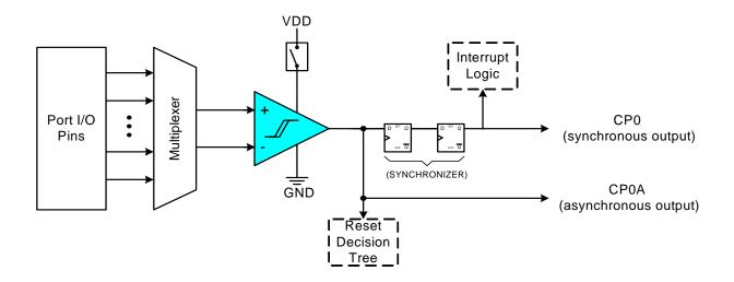
Figure 1.8. Comparator Block Diagram
