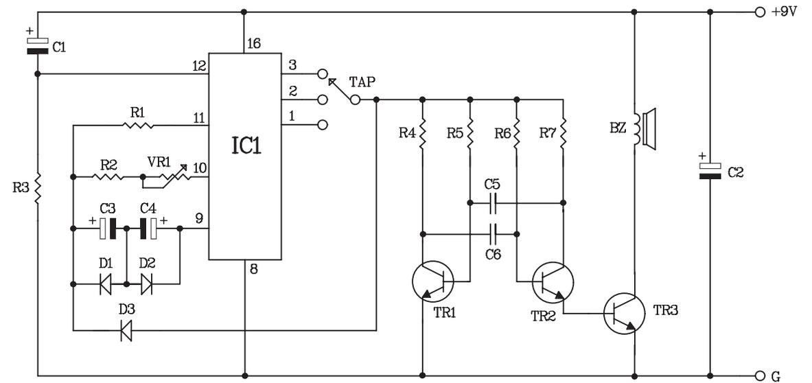
Figure 2. The alarm timer 1-240 min circuit
