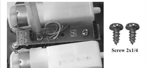
⑧ Mount BR002-1 PC-board into body robot and secure them with two #2 x 1/4" screws.
