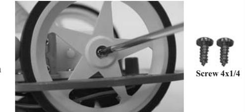
⑩ Mount sensor board into body robot and secure with two #2 x 1/4" screws.
