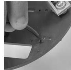
③ Insert the electric wire battery holder into body robot.
