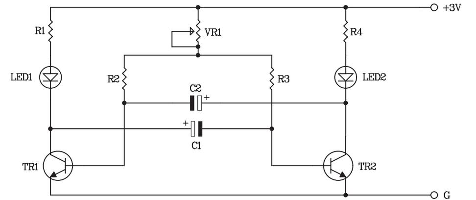
**Figure 2. JUMBO 2 LED FLASHER circuit**
