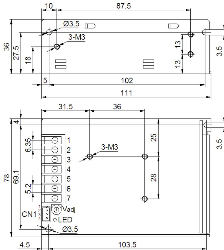
Length of assembly screw: max. 6mm
