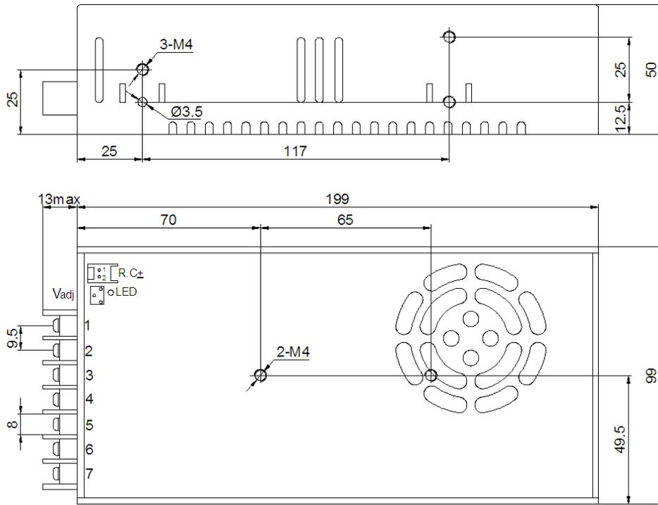
Length of assembly screw: max. 6mm
