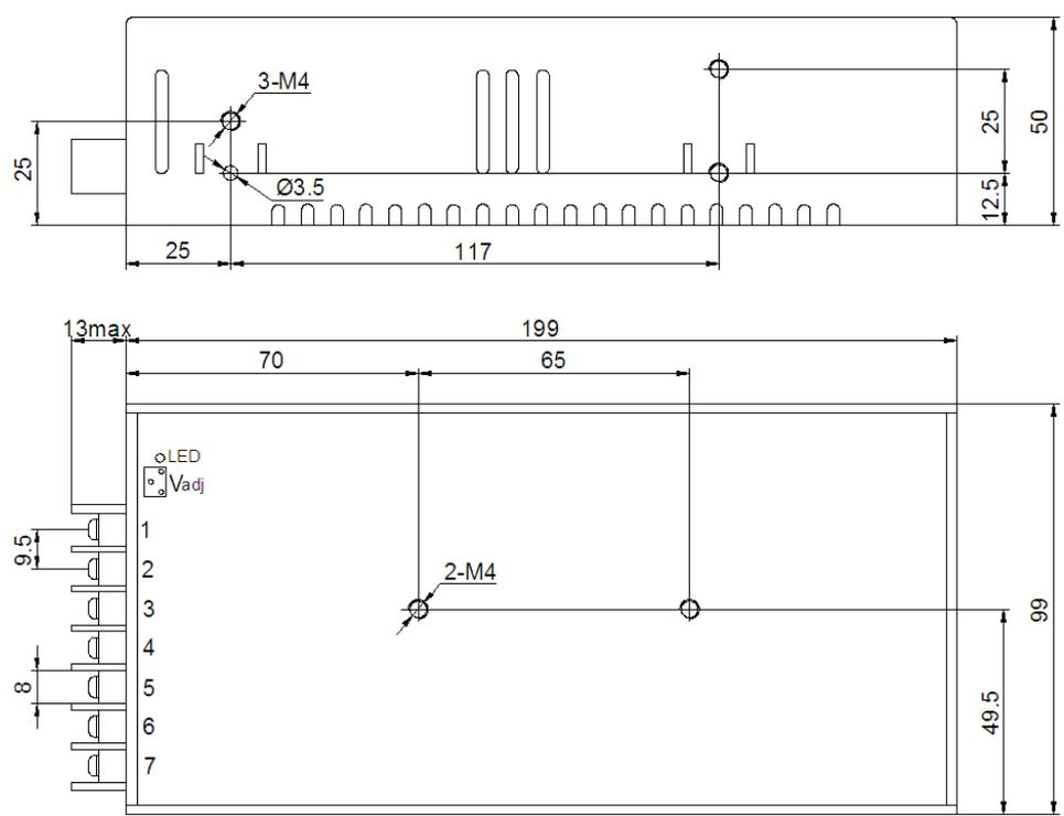
Length of assembly screw: max. 6mm
